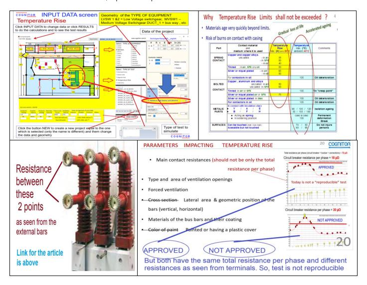
EXAMPLE OF IMPACT OF THE RESISTANCE OF THE CIRCUIT BREAKER IN THE BUSBARS THAT FEED IT Panel 1250 A – 1 bar per phase – temperature rise limit 75K – Copper bare bars.
