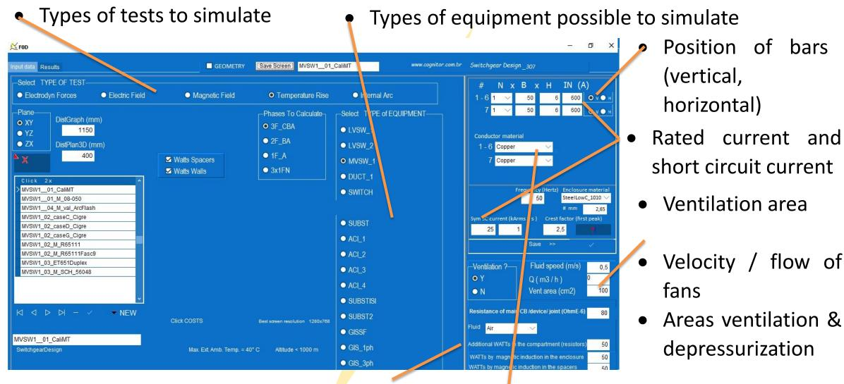
• Additional Watts ( for bus bars and connections are automatically calculated)
